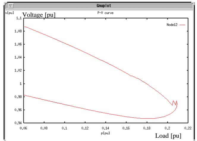
Fig. 4 A P-V curve of the optimal control (Node 12) for IEEE 14 bus system.
